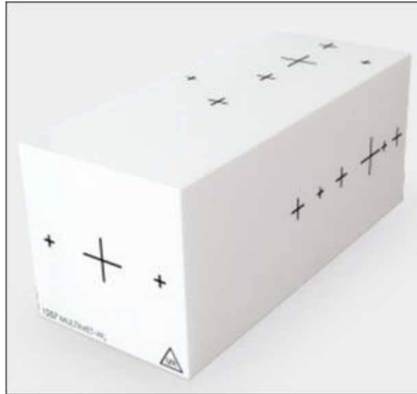
Figure 1 (b) Schematic of the MultiMet phantom
