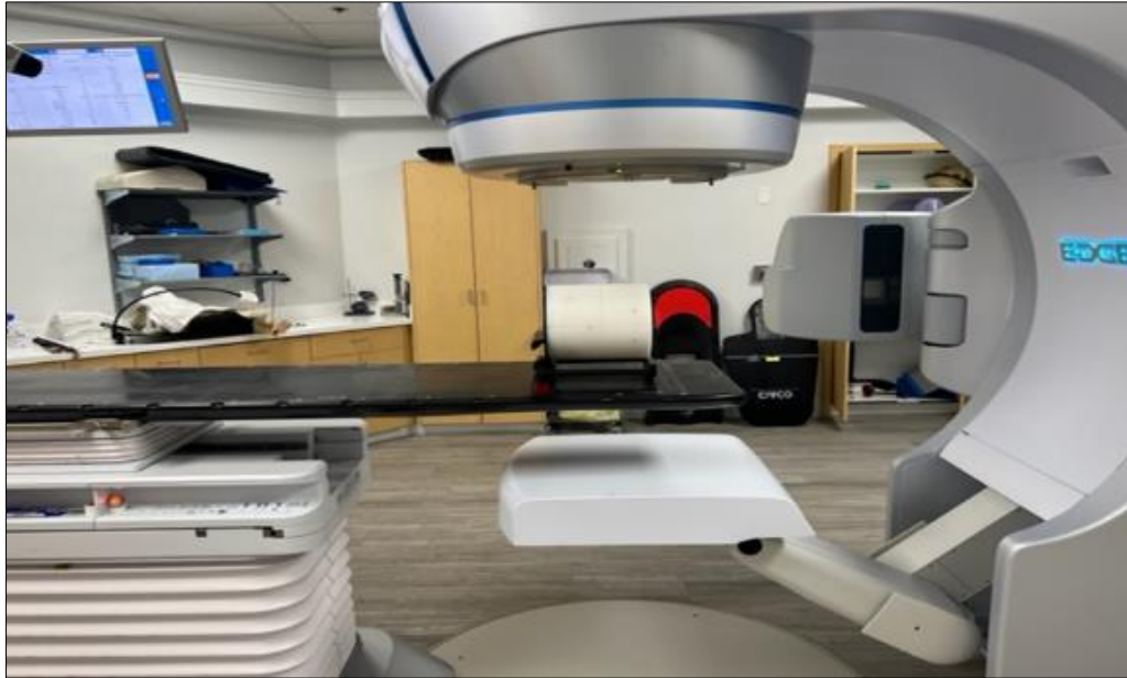
Figure 2 The Isocal phantom mounted to the couch during an isocenter verification test
