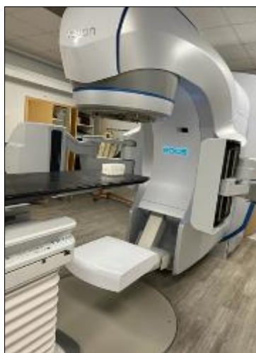
Figure 1 (a) Setup of the MultiMet phantom on the treatment couch with the machine reference at [0, 0, 0] coordinates
