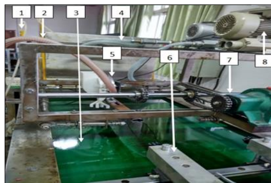
1. U-tube manometer; 2. Positive pressure line; 3. Greased belt; 4. Vacuum pressure line; 5. Metering device; 6. Oil supply device; 7. Variable speed motor; 8. Air pump.
