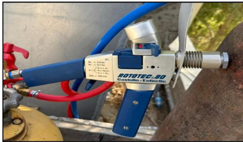
Figure 2: Photographic view of the commercial Rototec 80 flame spray torch utilized in the deposition process.
