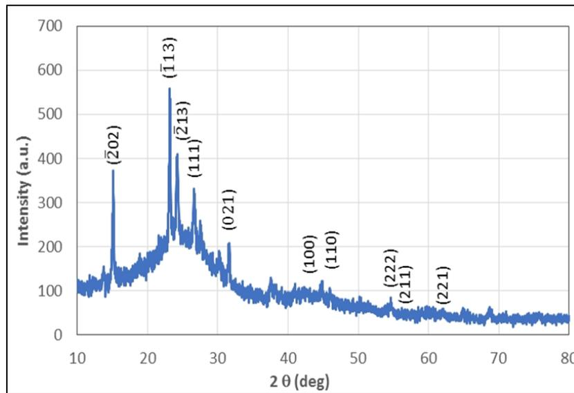
**Figure 3** X-Ray Diffraction Pattern of Gmelina wood Activated Carbon
