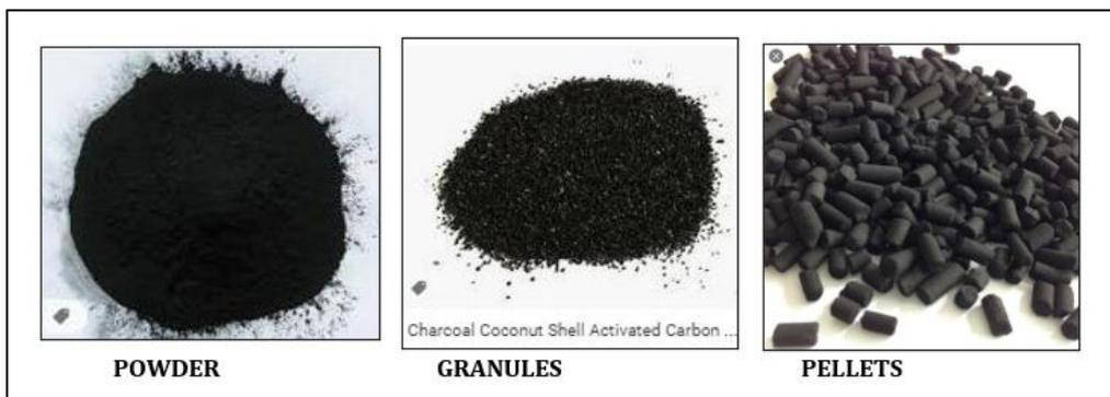
**Figure 1** Powder, Granules, Pellets Activated Carbon
